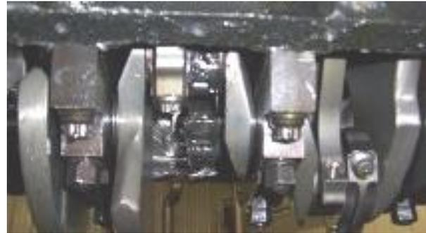
This crankshaft is galled, causing the connecting rod, center, to seize onto the crank and break off the end of the rod. Lack of oiling started this catastrophic failure.
