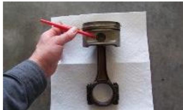
Mahle LT4 piston with GM powdered metal connecting rod. Wrist pins can seize to the piston if not properly lubricated.
